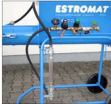
The water dosage armature is mounted at a comfortable working level and assures an exactly continuous mortar consistency
