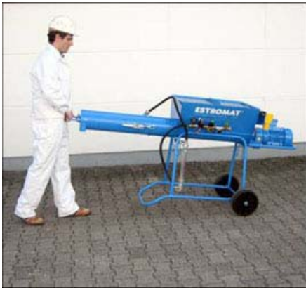
The ESTROMAT 404 continuous mixer can be moved at the site like a wheelbarrow.
