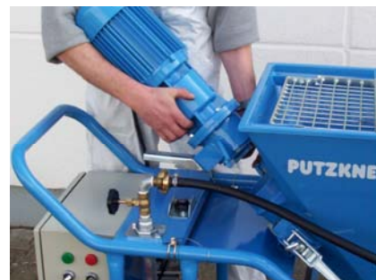
The pump motor is hinged away for cleaning the mixing tube. For transport the pump motor is removed.
