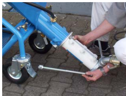
Above: Easily detachable pump part Left: The control module is removed for transport
