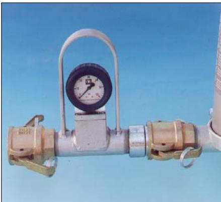
*The pump outlet is equipped with coupling SKM35 and mortar pressure gauge according to the safety rules of the German trade association.*
