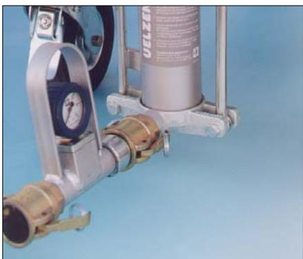
*The standard PUTZKNECHT S48-easy is equipped with screw pump parts UE4 silver and achieves 22 l/min. Depending upon application further conveying capacities from 5-30l/min can be obtained by exchanging the pump parts. Self-levelling screed work is possible with conveying outputs up to 50l/min.*
